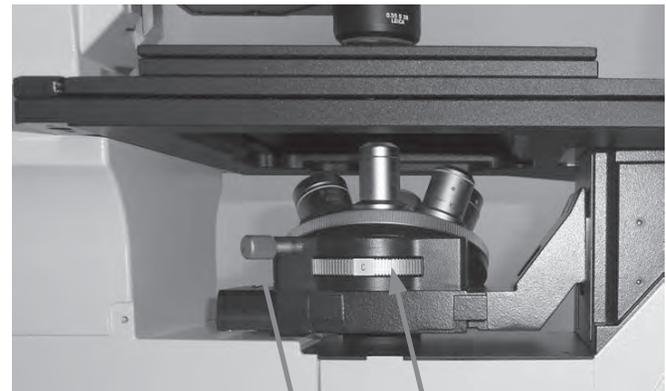
Fine adjusting the objective prism
