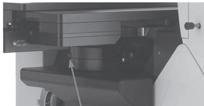
Fine adjusting the objective prism
