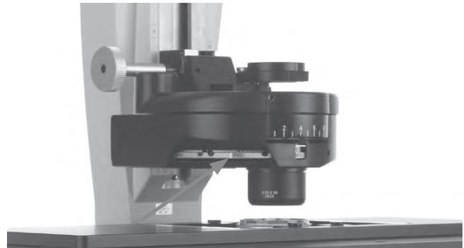
Condenser setting for tiltable Transmitted Light arm - configuring Darkfield stop (light ring)
