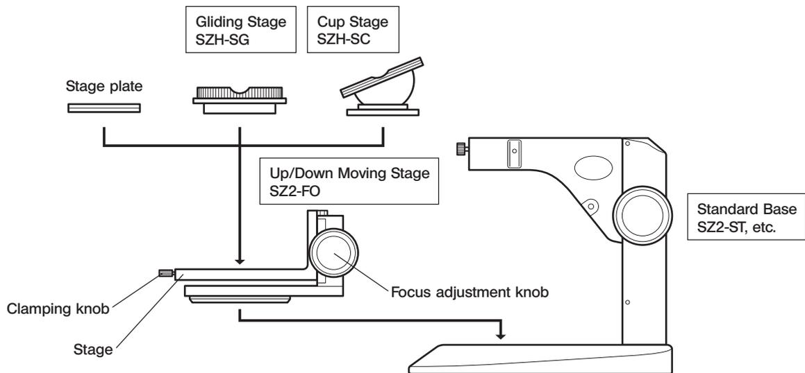
★ When using a filter or simplified polarized light system in combination with the transmitted illumination base, mount the filter holder or polarizer on the base before installing the up/down moving stage.
