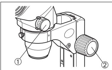
4. Set the zoom adjustment knob ① for the lowest magnification and rotate the focus adjustment knob ② to bring the specimen into approximate focus.
