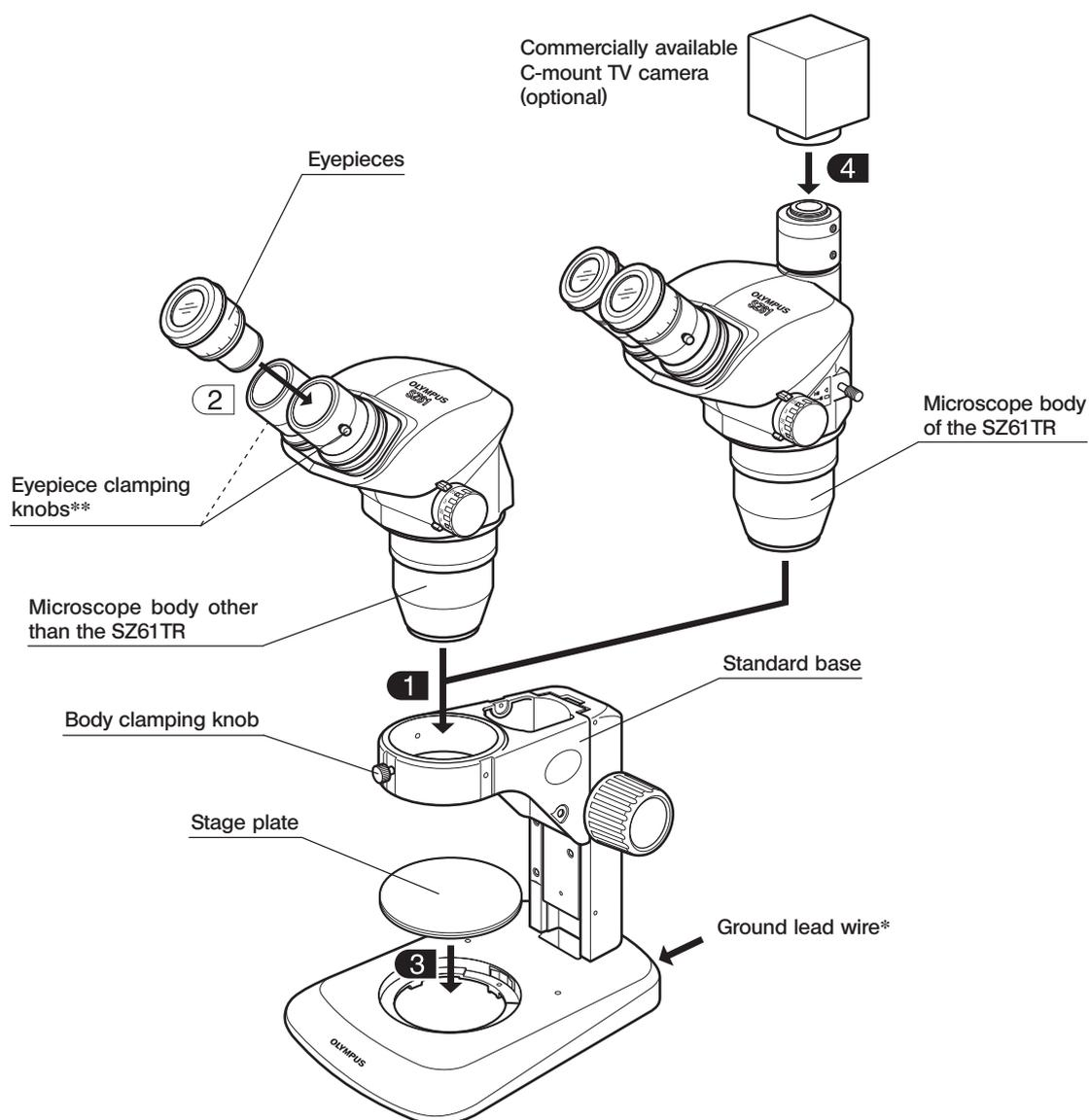
\* To reserve the ESD protection performance, be sure to ground the equipment using a grounding lead wire having a 4 mm banana plug.
