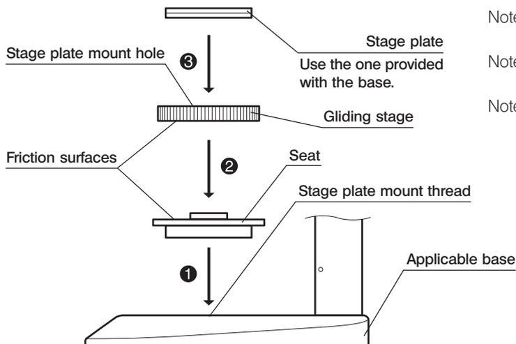
Note 1. Be sure to clean the friction surfaces if dirt or metallic power is attached on them.
