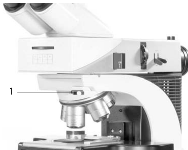
Fig. 64 Objective prism slide 1 Fine adjustment
