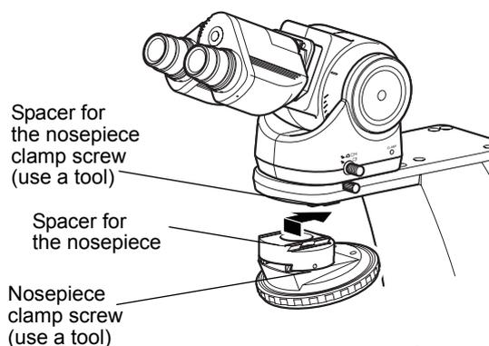
Attaching the spacer for the nosepiece
