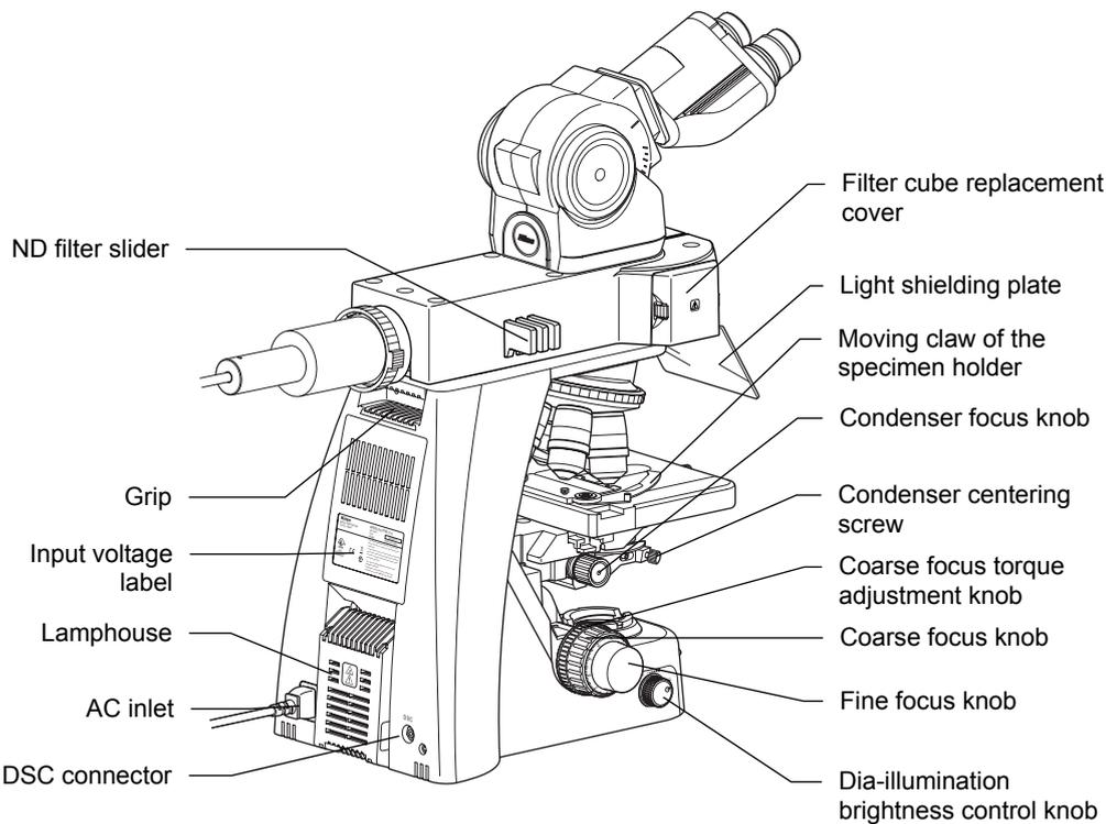
5.2 Epi-fluorescence Microscopy Procedure
