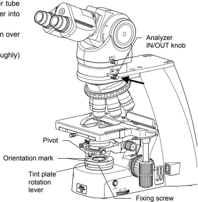
**Bringing the analyzer into the optical path
