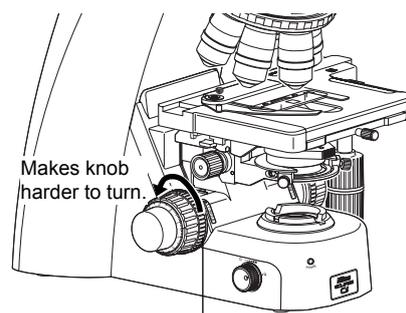
Coarse focus torque adjustment knob
