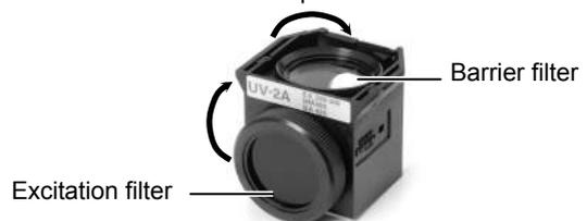
Replacing the excitation and barrier filters
