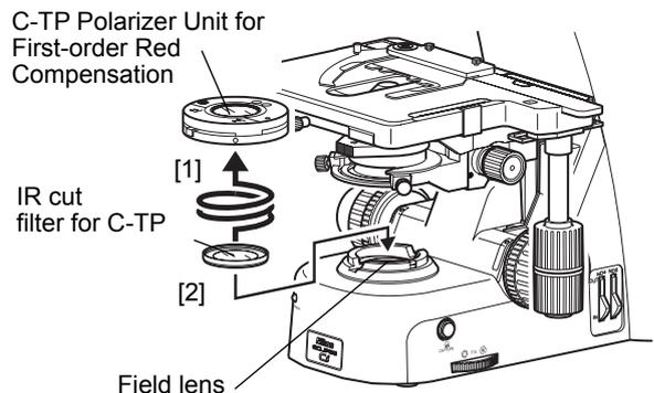
**Attaching an infrared ray blocking filter**
