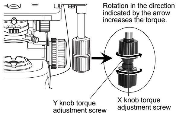
**Adjusting the torque of XY knobs**
