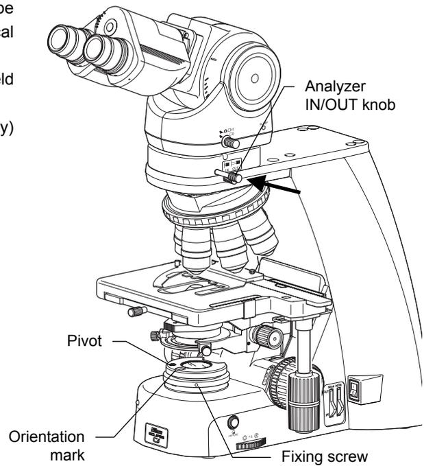
**Bringing the analyzer into the optical path
