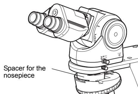
**Using the spacer for the nosepiece**
