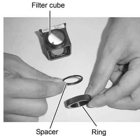
Attaching/removing the internal spacer
